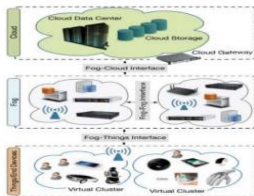
Figure 1: Architecture of Fog Computing (Atlam et al. 2018)
